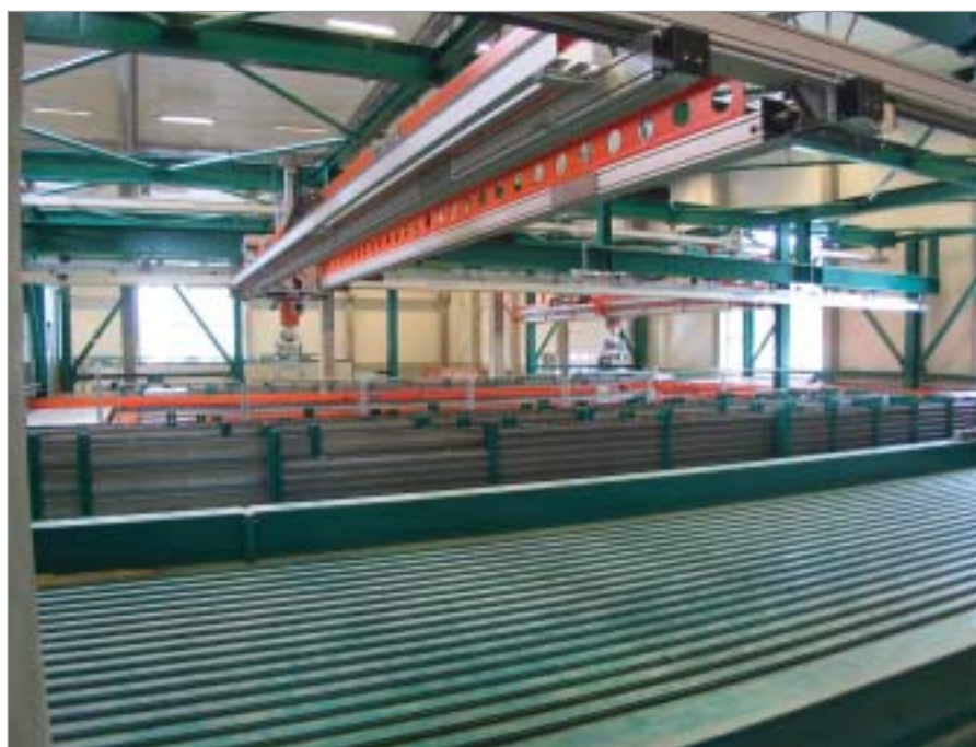
Magazine robot for solid-wall formworks
