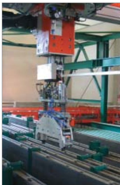
Magazine robot and formwork robot
