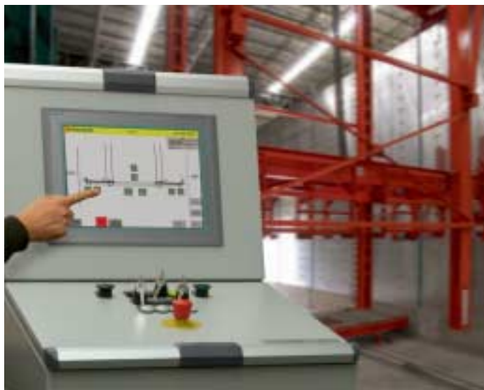
Fig. 1 Touchscreen for operating pallet rotation.
