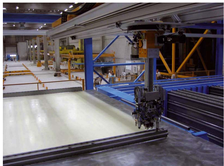
The formwork robot places the formwork following the application of the retarder
