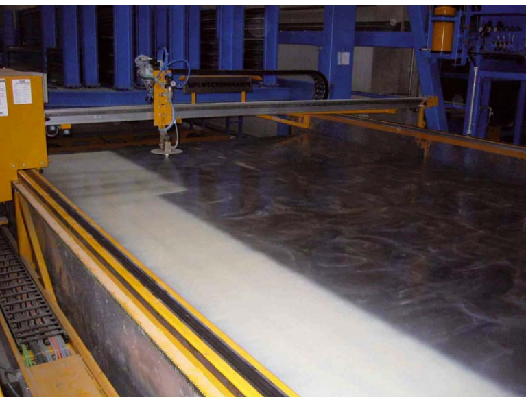
The coating robot sprays the retarder onto the pallet
