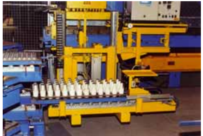
The shuttle ensures short travel paths of the insert robot
