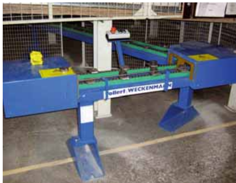
Feed belt for the electrical back box magnets
