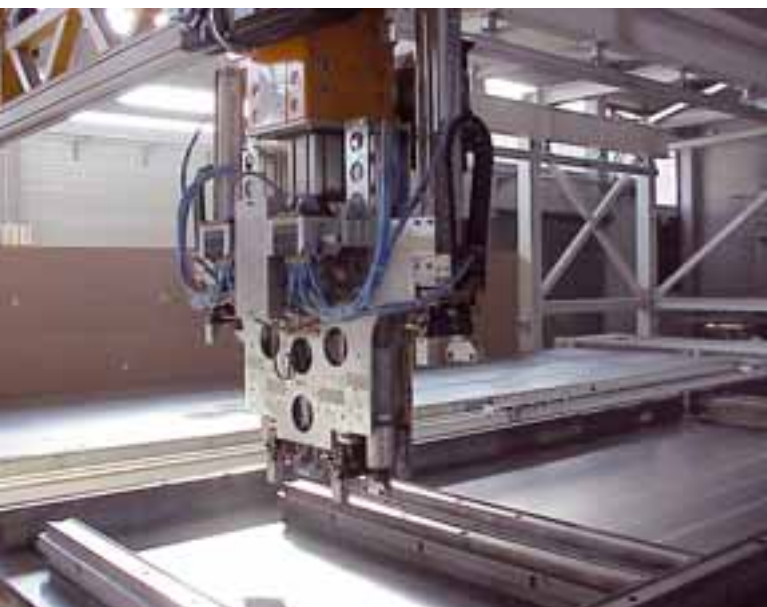
Weckenmann formwork robot with quadruple external gripper
