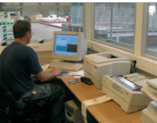
Control room with UniCAM central computer at Skandinaviska Byggelement in Sweden.
